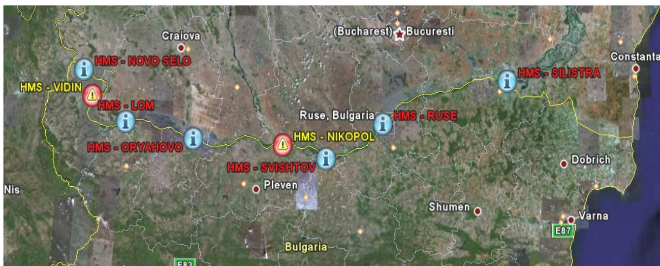
Figure 1 - Network of the hydrometeorological stations along the Bulgarian section of the Danube
