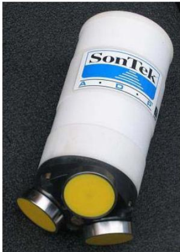
Fig. 4 The SonTek/YSI ADP (Acoustic Doppler Profiler)
