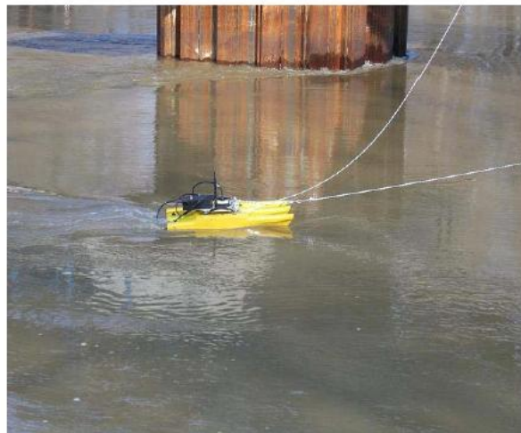
Fig. 4 The SonTek/YSI ADP (Acoustic Doppler Profiler)
