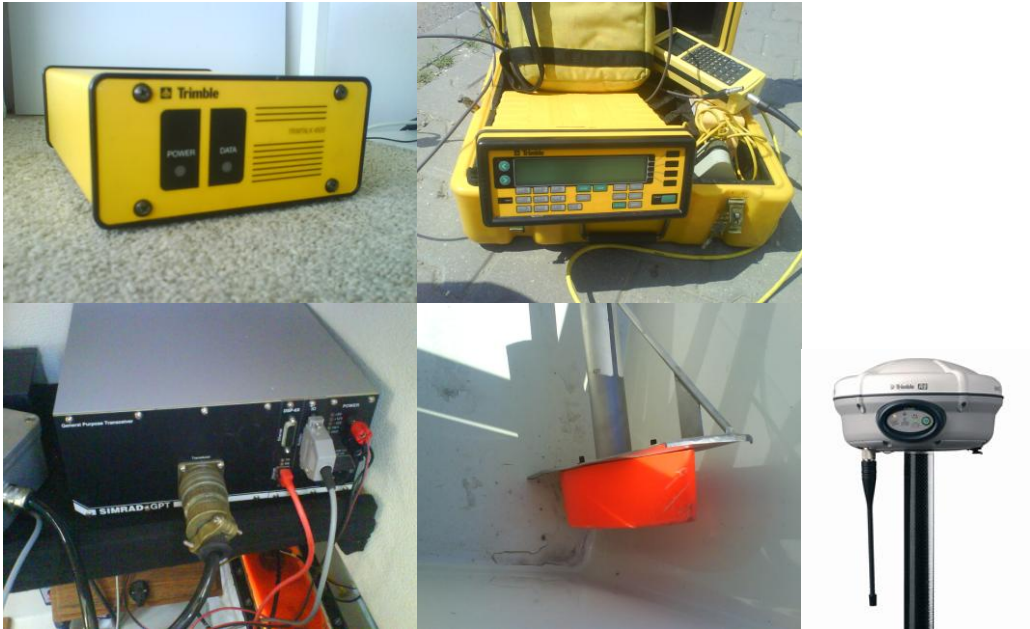
Fig.4: measuring system for sounding (base, echo sounder, transducer, GPS Trimble)
