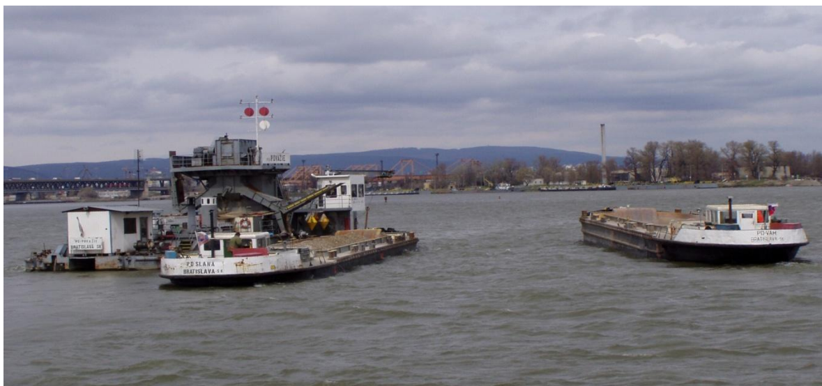
Fig7.: Transport of excavated material by motor pontoon barge
